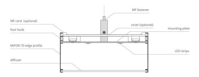
2. The maximum width for linear lighting fixtures with gentle curves is 300 mm. The above limitation results from the diffuser bending (hanging) when it creates a larger surface.
