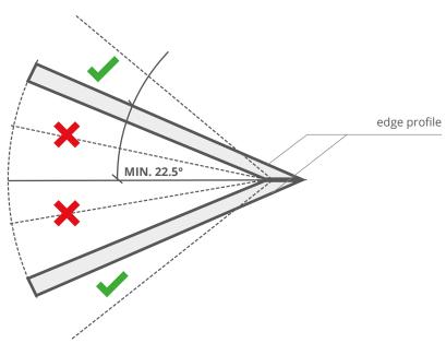
7. The minimum straight section in the edge profile necessary for easier installation of ZM connectors.
